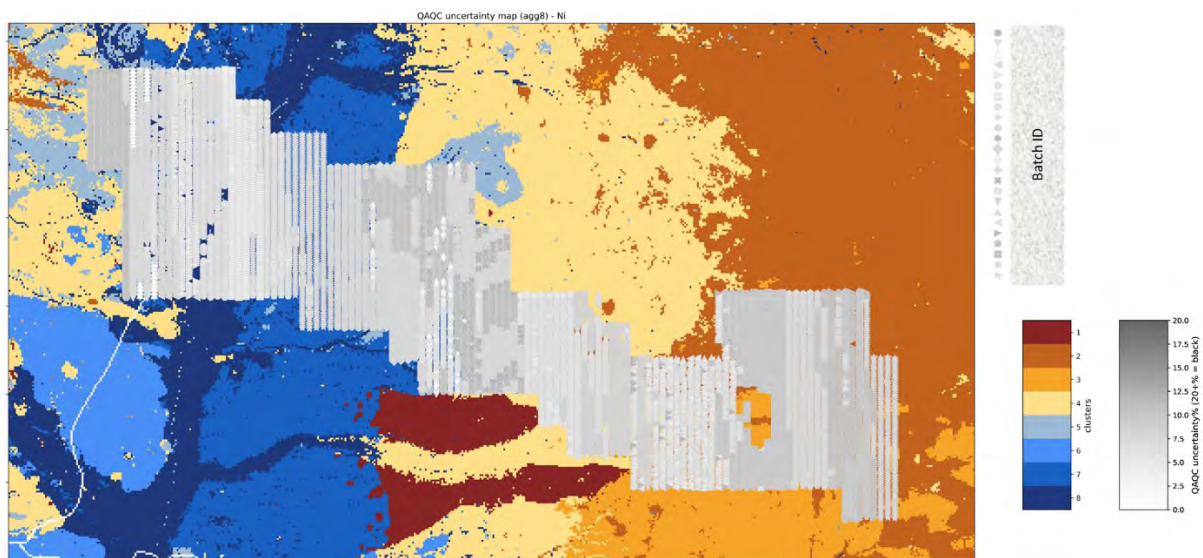
Figure 8: Example of a batch uncertainty map for Ni analyses over 24 different batches in a de-identified project area. Note that the batch uncertainty was based on duplicate samples to assess the combined precision of field sampling and laboratory analyses.
