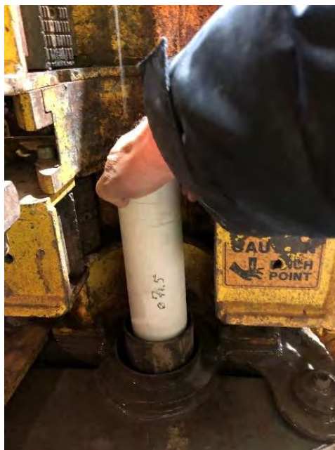
Figure 9. Driller-deployed cartridge containing tracer particles being deployed at the Kapunda drill site.
