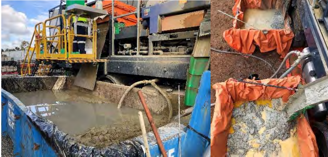
Figure 11. (Left) Solid waste collection in a single skip during drilling at Kapunda. (Right) Double skip waste collection from shale shaker (top of image) and centrifuge (bottom of image) during drilling at Delamerian South (Alawoona).
