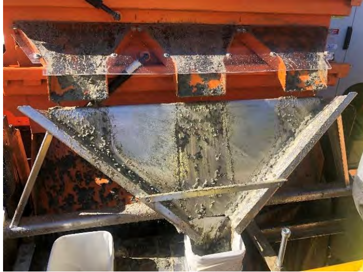
Figure 8. Coarse fraction cuttings discharging from the shale shaker into calico bag at the coarse fraction sampling station.
