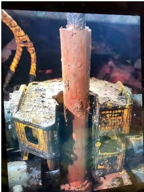
Figure 22. Sticky clays attached to the coil tubing and closing the entire annulus at the drill collar. This material contributed to sample system overload, causing blockages in the fluid splitter and sample shaker.
