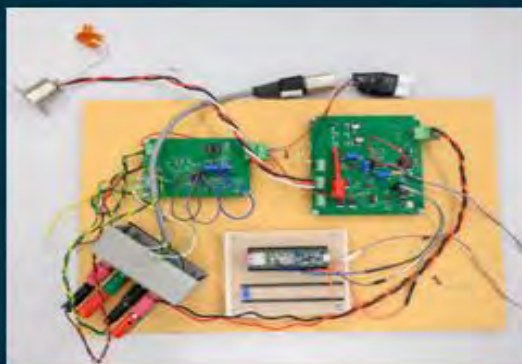
Rudimentary design stages of the downhole swept Frequency EM tool.
