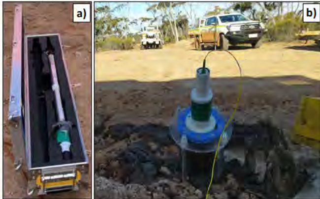
Figure 1 a) FLI probe in a case; b) FibreLine Intervention tool – a landing holder/plate on top of the bore and connected to an interrogator at the surface, probe deployed into the borehole.
