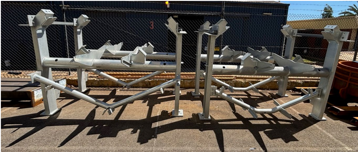
Figure 3: First commercial production run of ground modules with 508 mm rollers integrated.
