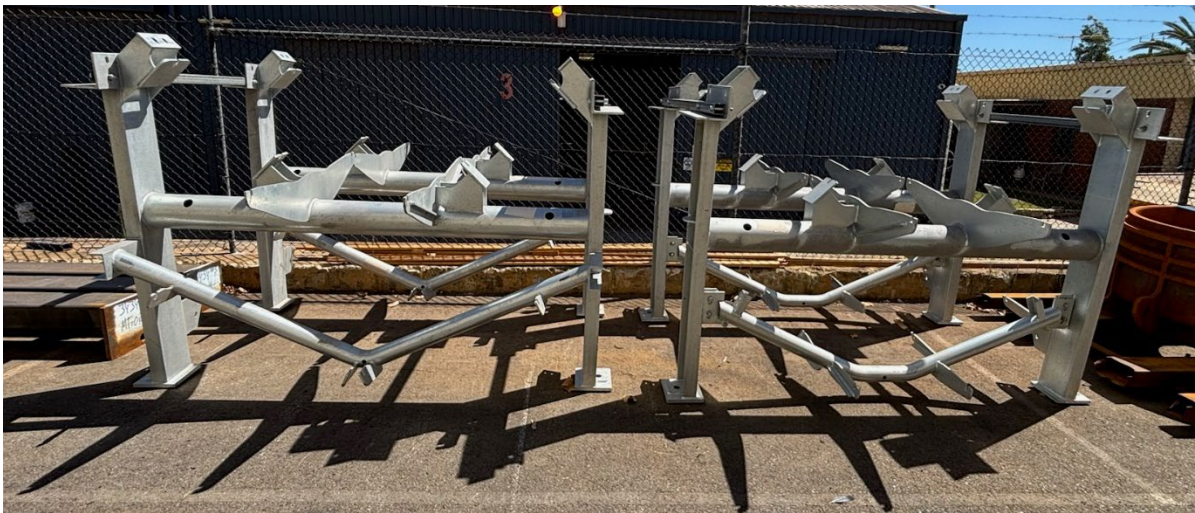
Figure 25: First commercial production run of ground modules with 508 mm rollers integrated.
