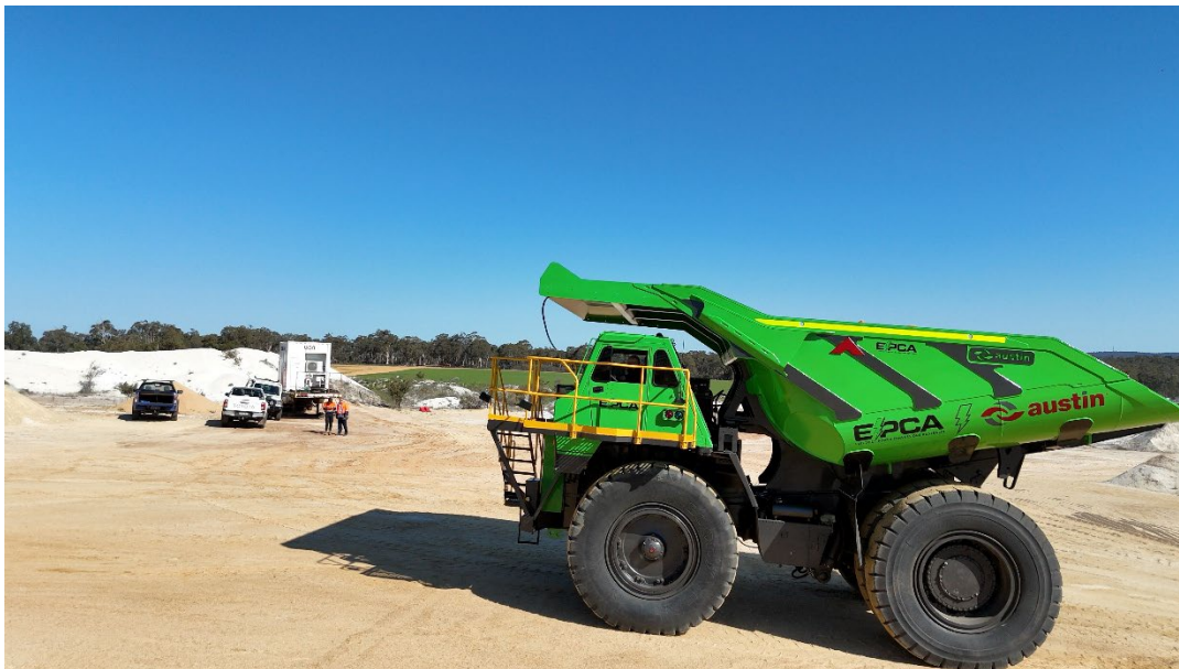
Figure 22: EPCA's E-777D-OHT Truck Being Tested at Bakers Hill
