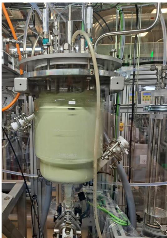
Figure 16 An 8 L reactor in batch mode with the overflow port blanked
