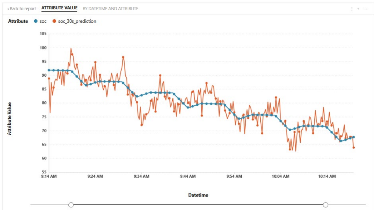
Figure 20: SOC Prediction - 30 Seconds Ahead.
