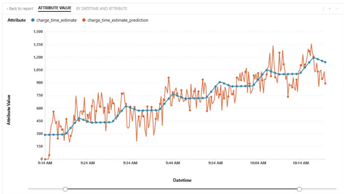
Figure 13: Charge time estimate model prediction for test session 1.
