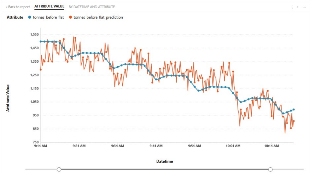
Figure 16: Total Tonnes Moved Before Battery Flat for test session 1.
