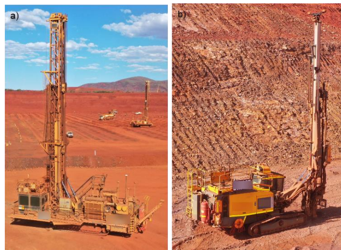
Figure 1. Representative drilling rigs employed in the collection of MWD data: a) Terex SKS 12, utilized for the drilling of 0.229m production blast holes and b) Epiroc D65, used in the creation of 0.165m wall control blast holes.
