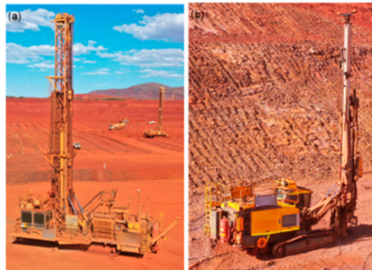
Figure 1. Examples of blasthole drill rigs used for collecting MWD data [52]: (a) Terex SKS 12, utilized for the drilling of 0.229 m production blast holes and (b) Epiroc D65, used in the creation of 0.165 m wall control blast holes.
