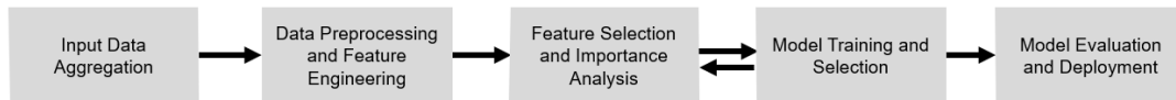
Figure 2.1 Analytical framework for MWD-based subsurface characterization. Feature selection and variable importance analysis can occur before and after model training, allowing for an iterative workflow in which modelling outcomes inform subsequent feature refinement.
